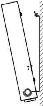
**2** Bring the radiator towards the mounting bracket and up, then insert the mounting bracket in the 2 wall brackets provided for this purpose.
