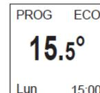
For example: for Monday you programmed a Comfort temperature period from 17:00 hrs to 23:00 hrs. You return at 15:00 hrs and the appliance displays an Eco temperature.
