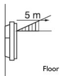
Detection is not possible underneath the sensor.
