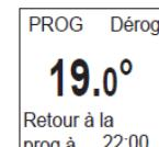
One-off bypassing of the programming is active up until the next Comfort temperature period that is defined in the program. The appliance then reverts to its normal operation.
