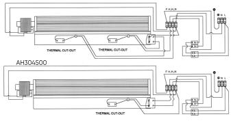
Both of these units are suitable for remote control operation, with the use of remote control switch part no. AH303005 shown in the diagram below
