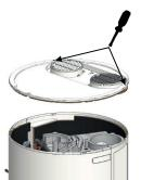
3. Unscrew the 2 rear screws on the top and then unclip it.
