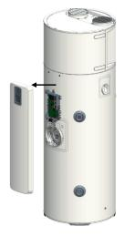
Lift the column off the inserts at the bottom, paying attention to the control screen cable and the earth cable.
