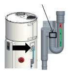
Please note: this operation must not be performed when installing in an ambient environment. For a ducted product, the full siphon is used to check the compliance of the ducting on the intake side.
