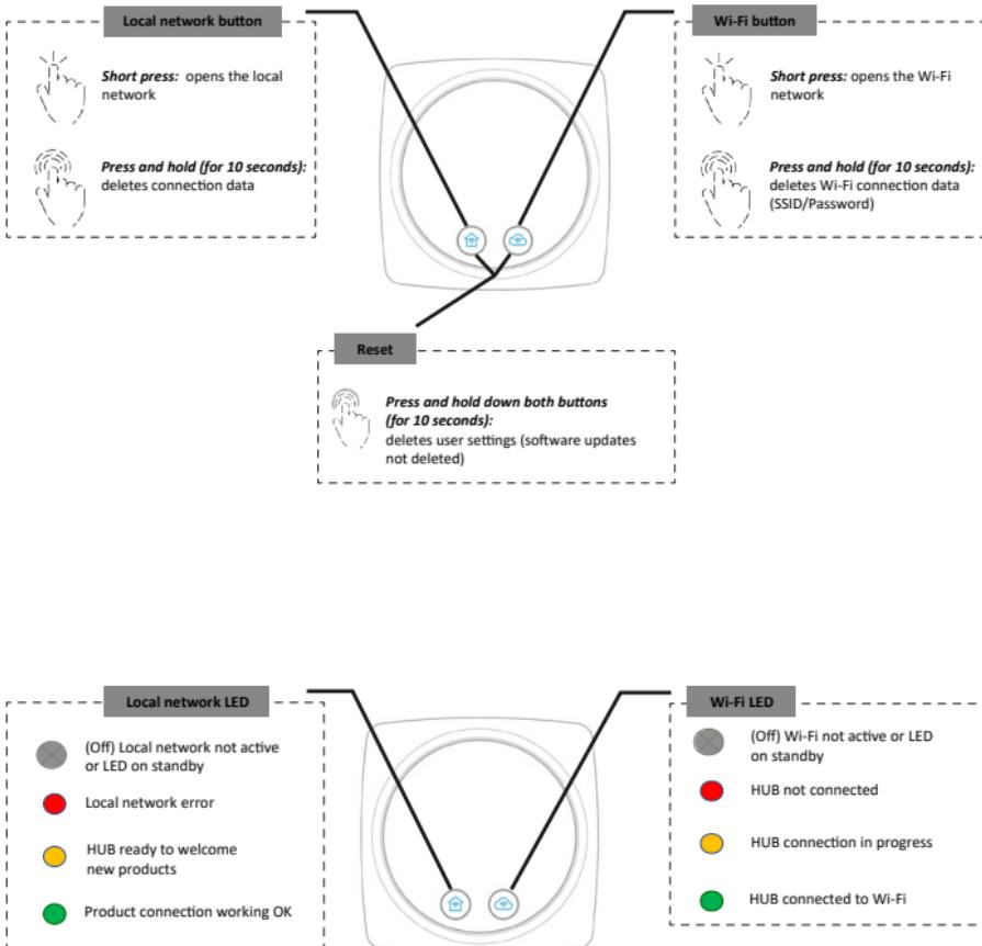
After 5 minutes of inactivity, the LEDs go out. The hub is on standby. Press a button to exit standby mode.
