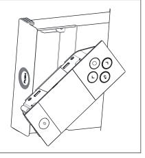
• Reposition the front part in the rear part of the control panel.
