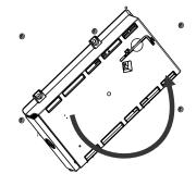
**9** Mount the panel bracket using the 4 screws.
