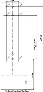
•Before screwing, align the bottom wall bracket marks with the 2 screws.
