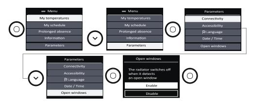
When the function is active, and the appliance detects an open window, it displays the following message:
