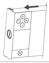
• Remove and keep the two mounting screws on the rear part of the control panel.
