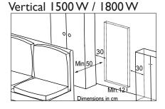
To optimise the presence detection of your appliance, avoid installing it in a tight corner, or behind a piece of furniture.
