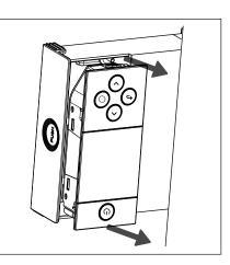
Swivel and screw back in. Reverse the direction of the panel cable and refit it.
