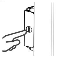
**6** Pull on the side of the panel so that it is completely visible.
